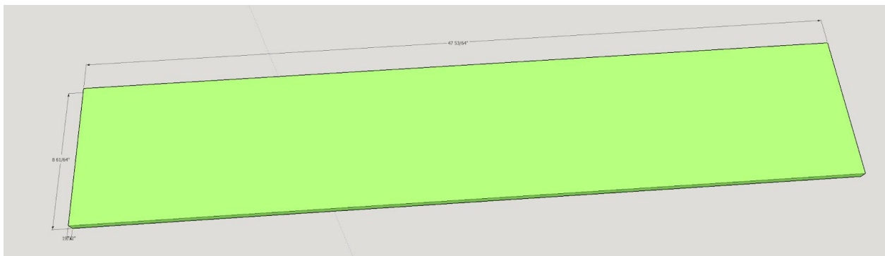
Top for back cabinet (this will need cutouts for the T-tracks if you use those).
